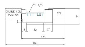
The coil itself can be rotated in 90° steps by releasing the four securing screws. (FIG 3) When rotating the coil care should be taken to ensure the core assembly (core, spring, seal and washer) remains intact and aligned correctly. This is easily achieved by only lifting the coil the small amount required to clear the screws enabling the coil to be rotated.
