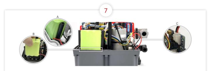
Place the battery pack (Element C) on the lower battery support (Element B) (Fig.7B). The battery cables should remain on the bottom part. Put the cables, as shown in the picture (Fig.7A). Connect the battery cables to the BSR PCB (Element A), as per (Fig.7C).
