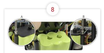
Place the upper battery support and fix it to the columns of the lower battery support (Element B), by using the Plastic fixing screws (Element F).
