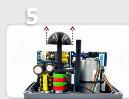
Carefully remove the position indicator.
