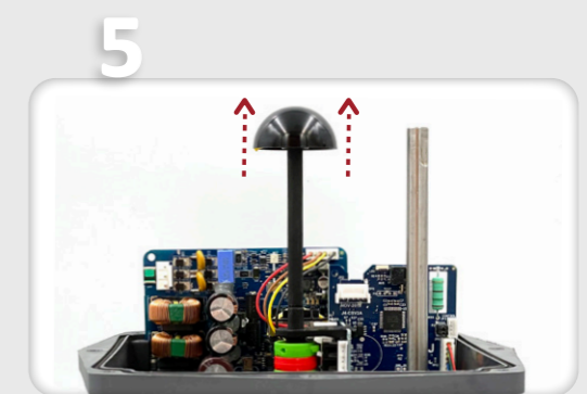
5 Carefully remove the position indicator.
