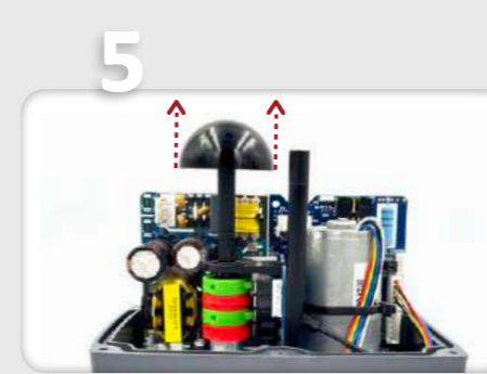
Carefully remove the position indicator.
