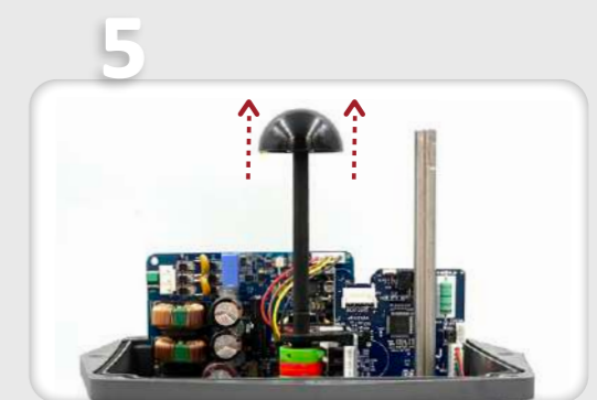
5 Carefully remove the position indicator.
