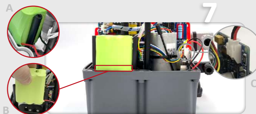
Place the battery pack (Element C) on the lower battery support (Element B) (Fig.7B). The battery cables should remain on the bottom part. Put the cables, as shown in the picture (Fig.7A). Connect the battery cables to the BSR PCB (Element A), as per (Fig.7C).
