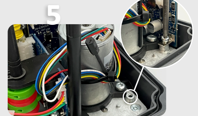
Fix it to the actuator metal plate, by using the Sheet metal fixing screw (Element E).
